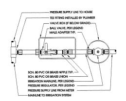
NOTE: ALL THREADED CONNECTIONS TO HAVE TEFLON TAPE OR PASTE.
