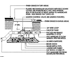
NOTE: USE 45 DEGREE ELLS TO ACHIEVE MAINLINE DEPTH FROM SUPPLY SIDE OF THE MASTER VALVE ASSEMBLY.
