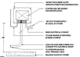
NOTE: INSTALL ENCLOSURE AS INDICATED PER PLAN & MANUFACTURER'S RECOMMENDATION. ROUTE WIRES AND SLEEVE THROUGH WALL TO RECTANGULAR PULL BOX AND TRANSTION TO DIRECT BURY WIRE.
