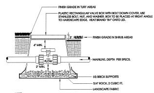
BOX TO BE INSTALLED TO ALLOW FOR PROPER OPERATION OF BALL VALVE HANDLE, INSTALL AT RIGHT ANGLE TO HARDSCAPE EDGE. INSTALL VALVE BOX EXTENSIONS AS REQUIRED TO ACHIEVE PROPER VALVE INSTALLATION AT MAINLINE DEPTH. ALL THREADED CONNECTIONS SHALL HAVE TERLON TAPE OR PASTE.
