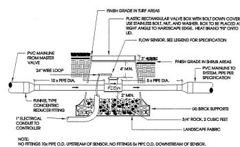
NO FITINGS 10x PPE O.D. UPSTREAM OF SENSOR, NO FITINGS 5x PPE O.D. DOWNSTREAM OF SENSOR, INSTALL FLOW SENSOR PER THE MANUFACTURER'S RECOMMENDATIONS, ROUTE WIRES THROUGH CONDUIT TO IRRIGATION CONTROLLER.
