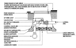
NOUS: ALL THREADED CONNECTIONS TO HAVE TEFLON TAPE OR PASTE. IF MARKLINE OR MANIFOLD SUB-MAIN IS AT VALVE DEPTH, TEE INTO VALVE WITH SCH.80 NIPPLE, LENGTH AS
